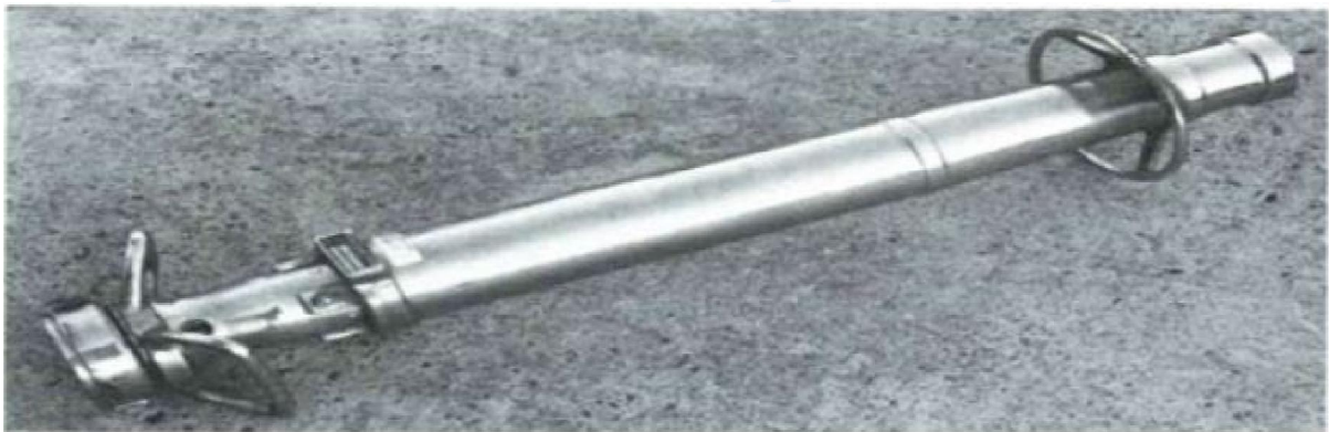
Figure 7.33 A typical hand-held foam nozzle.
