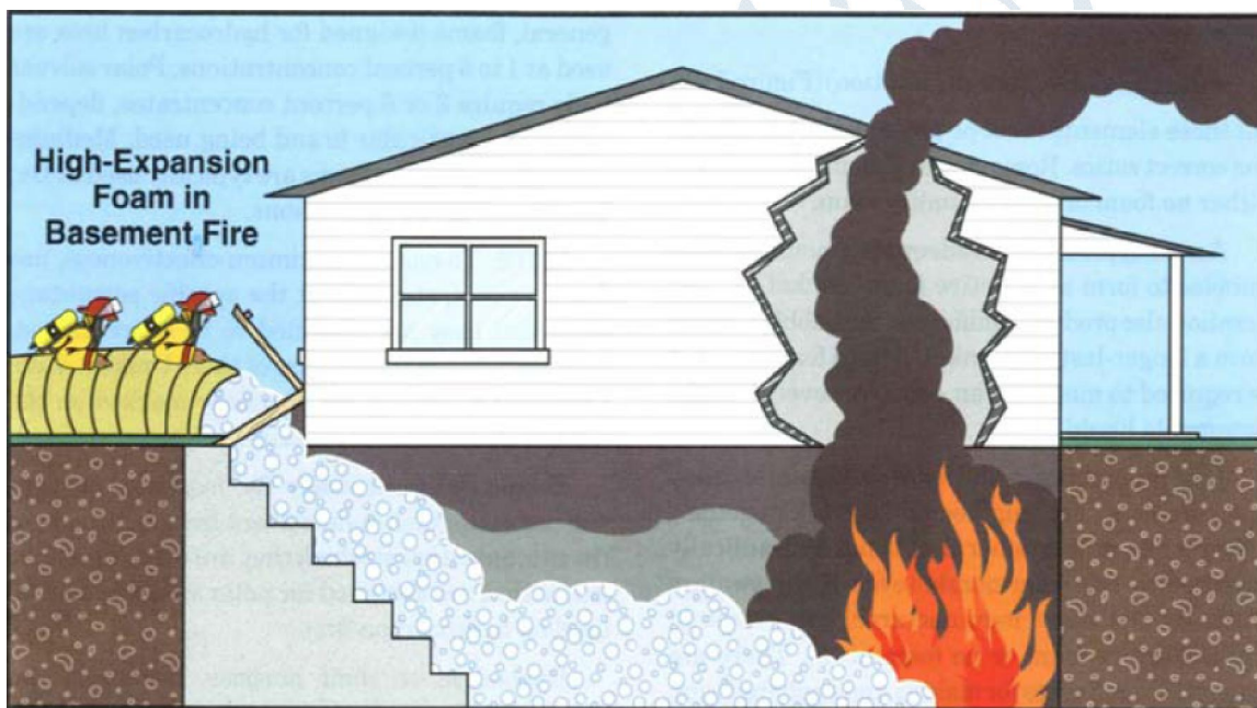
Figure 7.21 High-expansion foam may be used to fight hard-to-reach basement fires. Proper vertical ventilation tactics must be used in conjunction with this type of attack.
