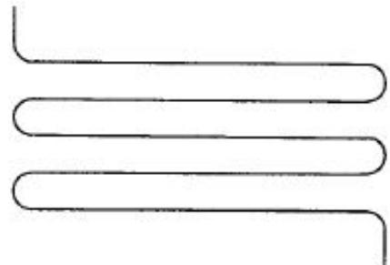
**FIGURE 13.24** Continuous pipe coil for radiant heating.
